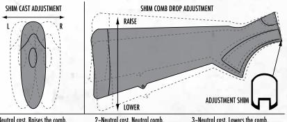
1-Neutral cast. Raises the comb. 1R/1L – Changes cast. Raises the comb.
