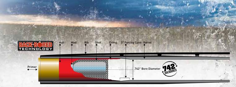
**BACK-BORED TECHNOLOGY** is based on extensive research and testing to find the secret to tighter, more consistent patterns. Instead of the traditional bore size of .729", this research shows the ideal 12 gauge interior diameter is .742". If the bore is any larger the gases will blow by the shot cup and reduce pellet velocity. If the bore is too tight the pellets are deformed as they pass through the forcing cone, causing poor ballistic performance.
