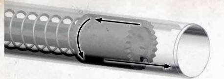
**SPEED-PLUG SYSTEM** lets you remove the three-shot adaptor with your fingers. Just remove the magazine cap, push on the spring retainer holding the spring in place, twist and remove the adaptor. It's a trouble-free design that lets you "pull the plug" in mere seconds without any tools.
